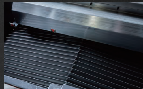
ベローズカバー仕様 (標準) 粉状の切粉の時に Bellows Cover Specifications (Standard): Designed for powdery chips to prevent their ingress.
